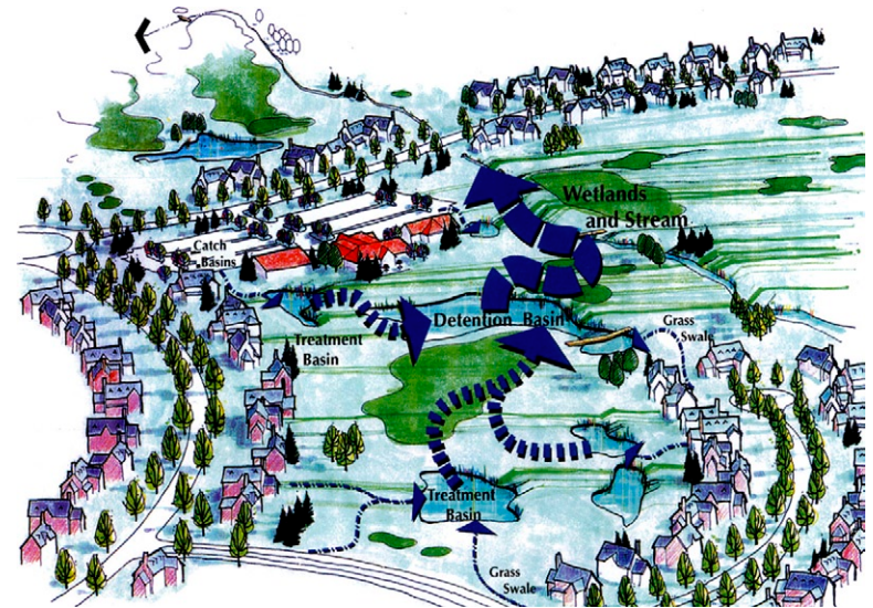
LID integrates open space with hydrology to filter stormwater
